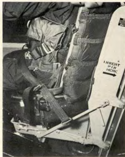
Parachute and survival kit attached, pilot has difficulty climbing out of A-1E/G seat.
