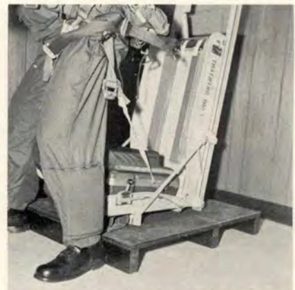
Plunger (arrow) is key to separation from survival kit. If it's extended when you pull secondary escape handle, you remain attached to raft (right).
