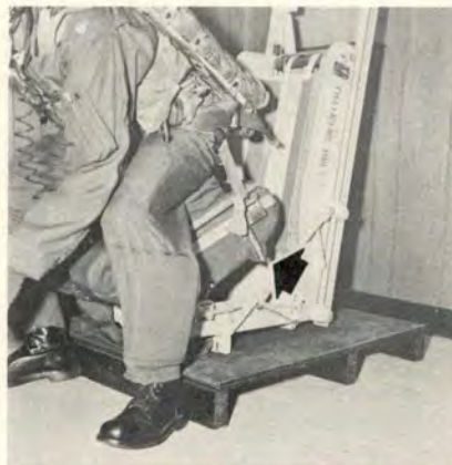
Plunger (arrow) is key to separation from survival kit. If it's extended when you pull secondary escape handle, you remain attached to raft (right).
